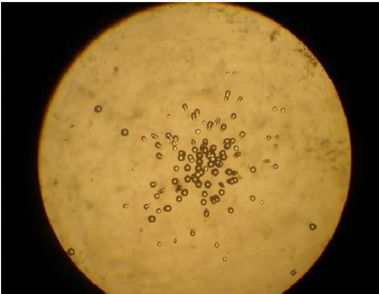
Figure: Microscopic round and oval pits in the surface of a plastic sheet of CR-39 (TASTRAK) burned by alpha rays from a micron-sized PMP some 10 micron above the sheet. Background counts are show by
